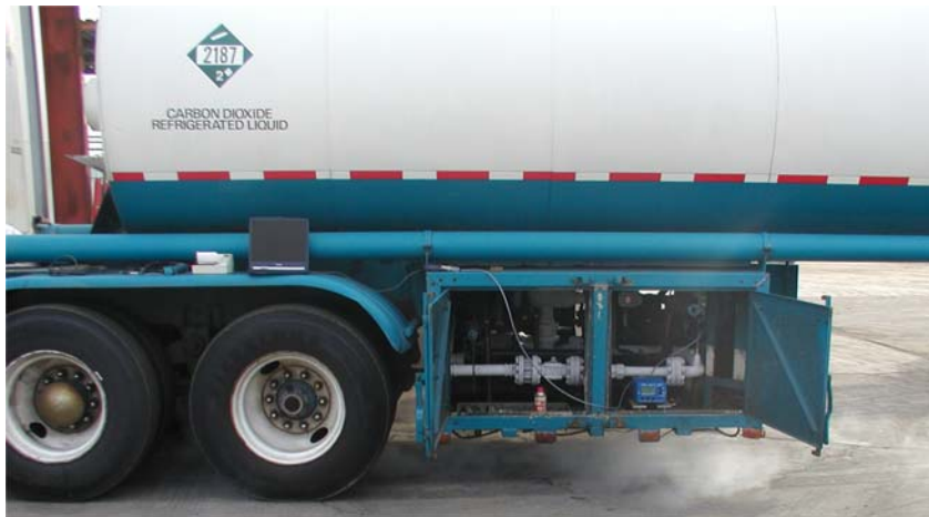
ACE II cryogenic system during testing on liquid CO2 truck application.
