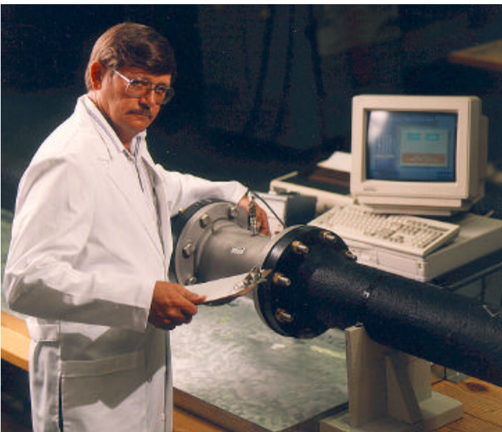
In house calibration facilities allow Hoffer to verify flowmeter performance for Sun Pipeline.
