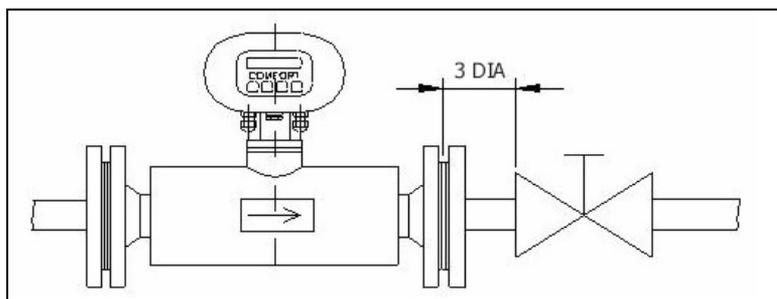
Required straight piping section for a “disturbance” located at the sensor output
