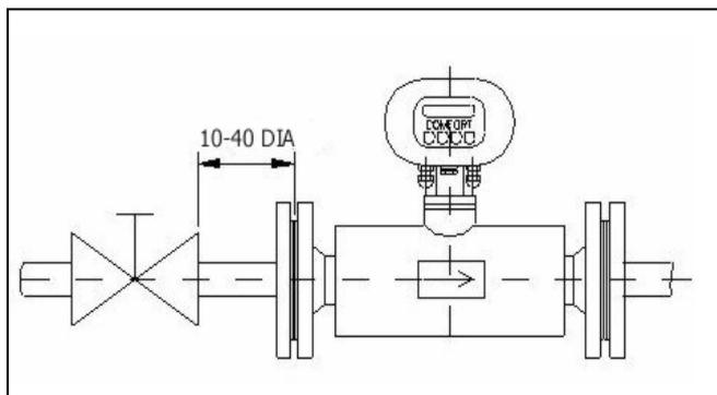
If any fluid-flow control element is located in the piping on the sensor output side, the sufficient length of the flow stabilization piping is 3 D.
