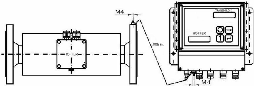
Earthing connection between the sensor and the electronic unit (the remote electronic)
