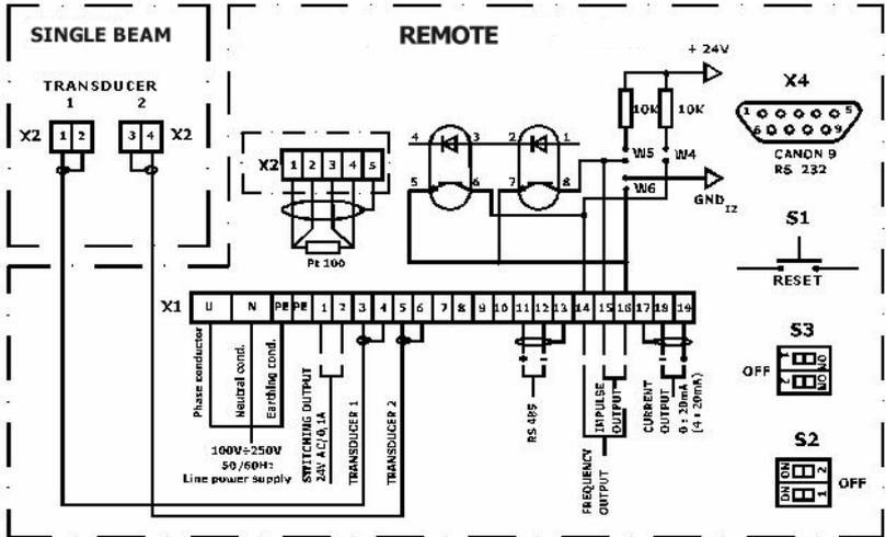
A remote electronic of flow meter with flow sensor DOUBLE BEAM
