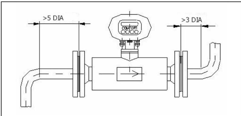
Required straight piping sections to stabilize the fluid flow through the sensor
