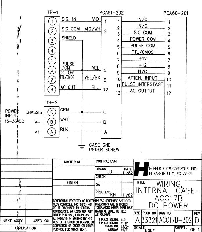
1. WIRE TO 7 OR 8 DEPENDING ON TYPE OF OUTPUT WAVEFORM DESIRED AND SPECIFIED.
